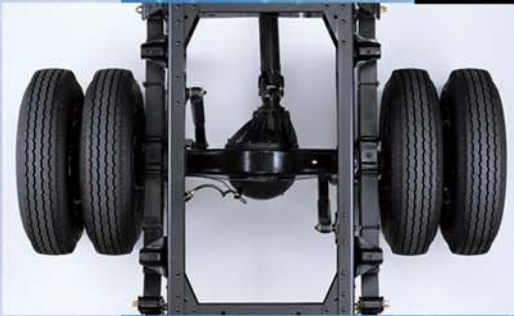
Under carriage - Bias shock absorbers to reduce vibration when getting under way. Eliminates rear wheel bounce when reversing up hill with no load.
