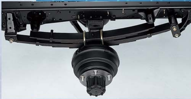
The leaf springs guarantee a satin smooth ride, an important consideration in the bus application.
