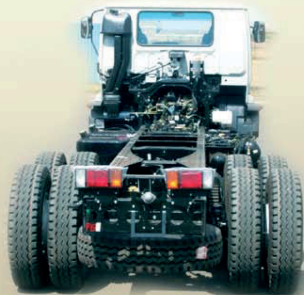
Heavy duty chassis on the 6 x 2 FVX
